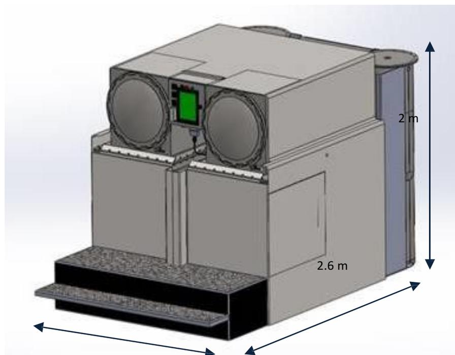
**Schematic of Micro Auto Gasification System (MAGS™)**
